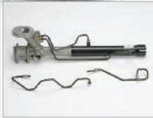
Power Steering Feed Tube
